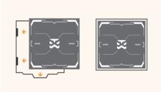
Ensure the base plate is clean & flat, and aligned with the platform.
